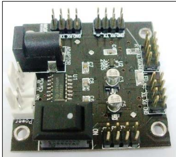
[Figure A-2a] RS-232 Communication Signal Adjustment Circuit Board
